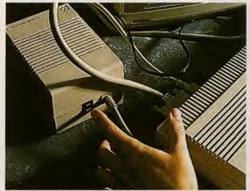
The A500 power supply is only guaranteed to power one extra disk drive. Some can do much better than that, but try potential purchases to make sure you have the power.
